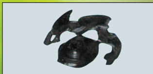
Impeller made of ordinary ABS resin After 24 hours of pump operation Loss of impeller weight:46%
